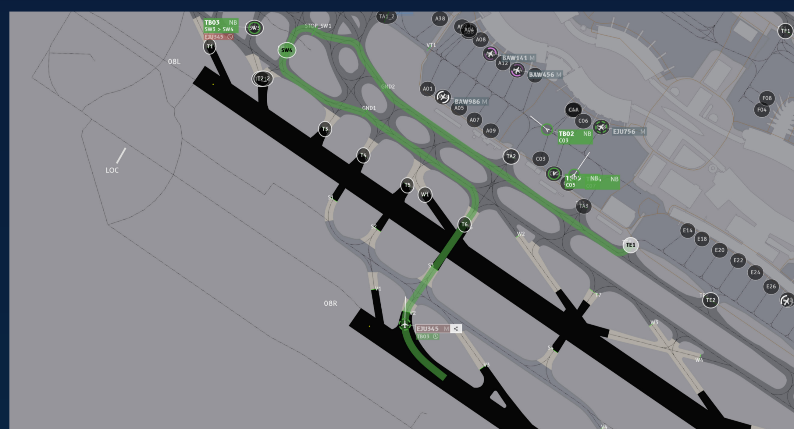
A-SMGCS HMI is completed with information on the taxi techniques and the routing service is updated accordingly.
