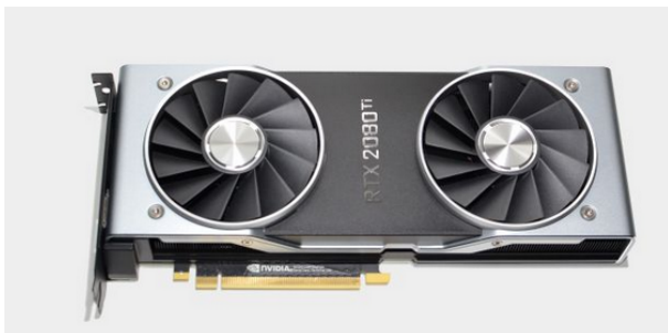
Figure: Nvidia GeForce RTX 2080 Ti, CUDA Cores: 4352, \simeq 30 TFLOPS ....
